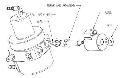
**INSTALLATION AND VEHICLE TEST**: Reinstall the regulator into the vehicle bracket. Tighten the inlet fitting to the regulator body; leave the outlet fitting to the regulator body disconnected from the outlet fuel pipe.
