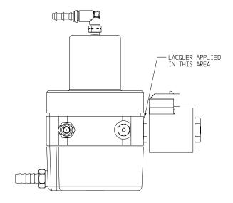
With the HPLO unscrewed from the regulator, remove the plastic retainer and seal. Use care not to damage the HPLO body cavity. Clean the regulator body HPLO cavity with compressed air.
